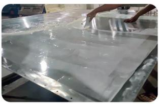
5. The panel is heated and pressed, to form a sandwich.
